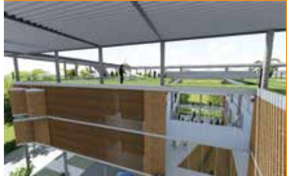
Perforated brick walls and opening for natural light and ventilation
